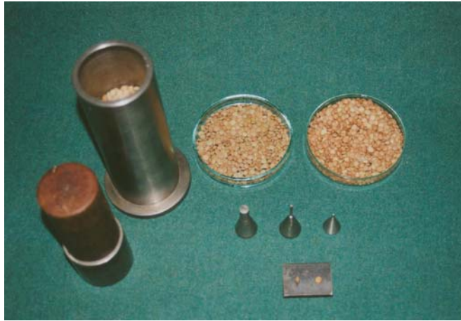
Photo 13. Preparation of material and equipment for the study of the mechanical properties of lentil seeds
