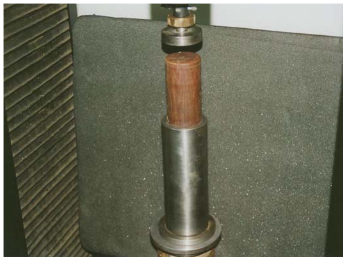
Photo 16. Stress relaxation test – cylinder placed in the „Instron” strength tester
