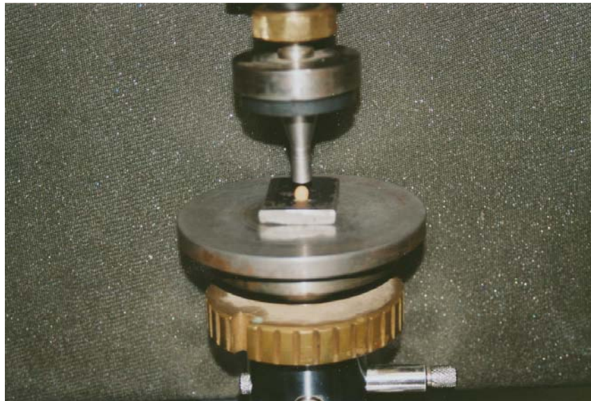
Photo 14. Single seed compression in the vertical plane
