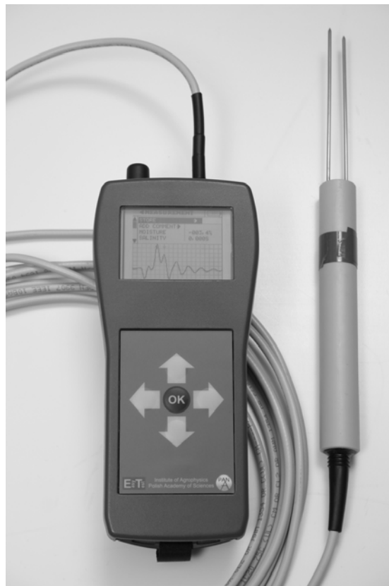
Fig. 58. Prototype of a handheld soil water content, salinity and temperature meter constructed with the application of modern components
