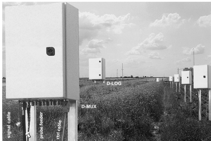
Fig. 59. An example of the D-LOG/10/mts-controlled stand incorporating six D-MUX/10/mts 2-nd level multiplexers. Maximum amount of the controlled FP/mts (or FP/m) probes is 60. For clarity only a single D-MUX was linked with the D-LOG and a single probe was connected to each D-MUX when taking the picture
