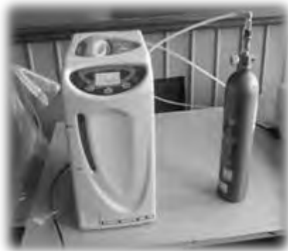
Fig. 1: The equipment structure for the hydrogen production and storage technology connected to Photovoltaic solar energy conversion system
